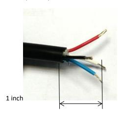
6. Remove the isolation from each wire for 5mm.
