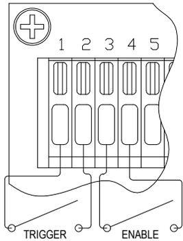
Closing the STANDBY inputs on TB-2 simulates the sensor STANDBY/RESET override. The user may close this momentarily to clear the delay off timer of a snow melt cycle. However, the user may also connect the leads of a toggle or wall switch across the TB-2 inputs to allow manual enabling and disabling of automatic snow detection. **Note that, if power is lost, the CDP-2 will always**
