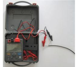
Each cable undergoes a 1,500-V dielectric insulation test in the factory as well as a conductor resistance test.
