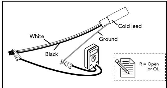
For the Full Limited Warranty to be valid you must perform the insulation resistance test using a megohmmeter (megger). In a two-step method, perform the above test at 500 volts DC and then at 1000 volts DC. Please record the readings on the Test Log Sheet.
