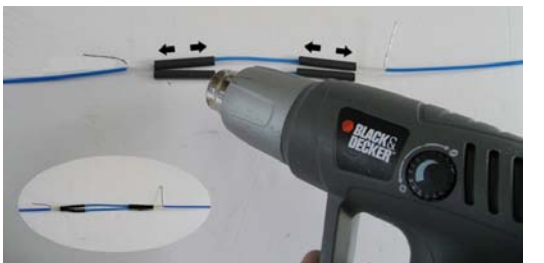
4 Center the 4 black heat-shrinkable tubes over the connectors and using the heat gun shrink in place
