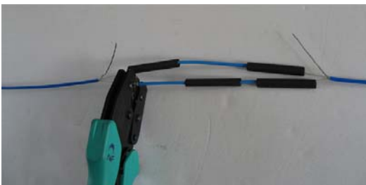
3 Using the crimp tool and connectors carefully connect the heating cables to the jumper wires and don't forget slide the heat-shrinkable tubes onto each jumper wire.
