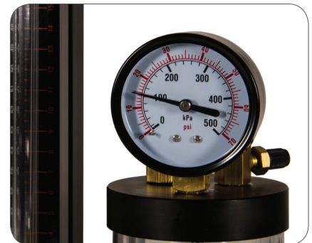
Dial gauge measures absolute pressure in kPa and psi.
