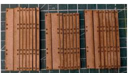
Gather all the interior columns as shown in the photos on the left. The interior columns are intended to hide the places where the exterior columns are inserted. You have three lengths of columns, the longest go to the top floor. Take care to glue them in the right direction since they are beveled on one of the two ends. The shortest columns (in the center of the photo) are glued to the middle floor and the right columns (those which are 7.5cm) go to the lowest floor.
