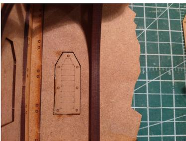
Finally, you can stick the cardboards in the openings of the windows. I recommend using CA (Cyanoacrylate) glue and only do the outline as shown. White glue contains a lot of water and tends to warp the cardboard.
