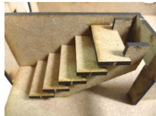
Glue the stairs into the floor's slots and insert part [T] along the wall using the remaining slots on both parts [S]
