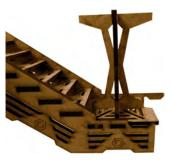
Glue one foot (assemblage of [A and B]) under the platform [R]
