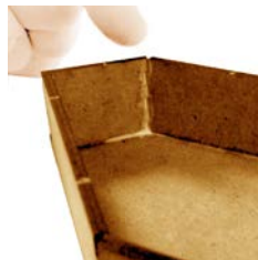
Apply some extra glue on the corners' interior
