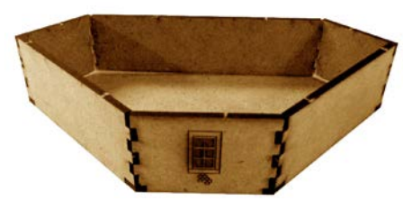
Spread glue and insert part [14] to close the back. Apply additional glue in the corners' interior
