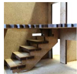
You will notice that the [B17] parts are wider than the [B16] and this is normal. The aim is to allow you to insert part [B17] into the wall to solidify the stairs.
