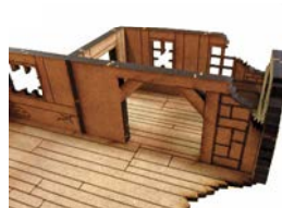
The assemblage of [H] and [H1] fits into the two holes in the floor, near the house's entrance. Make sure that the plain side is close to the wall [E1]
